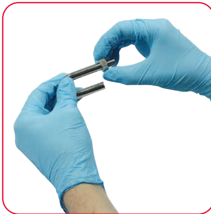
2. Install nut on the new Pigtail. NOTE. Pigtail should be installed with Loctite® 270.
