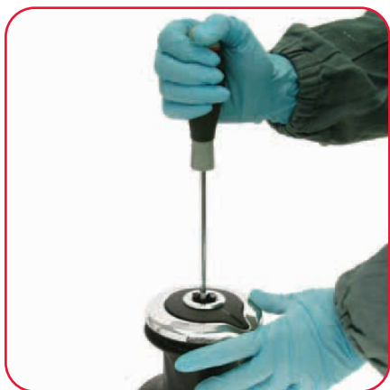
1. Unscrew the central screw (2Nm/18in-lb)
