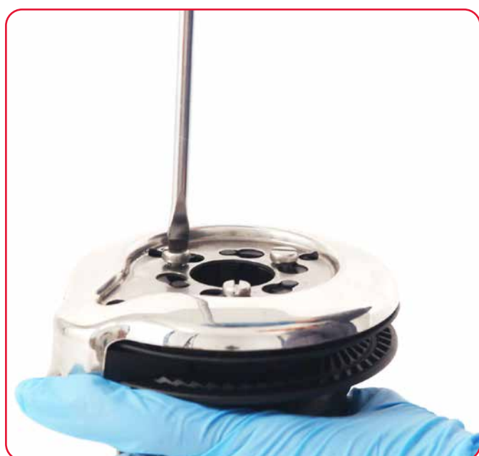
3. Unscrew the three screws (4Nm/35 in-lb).
