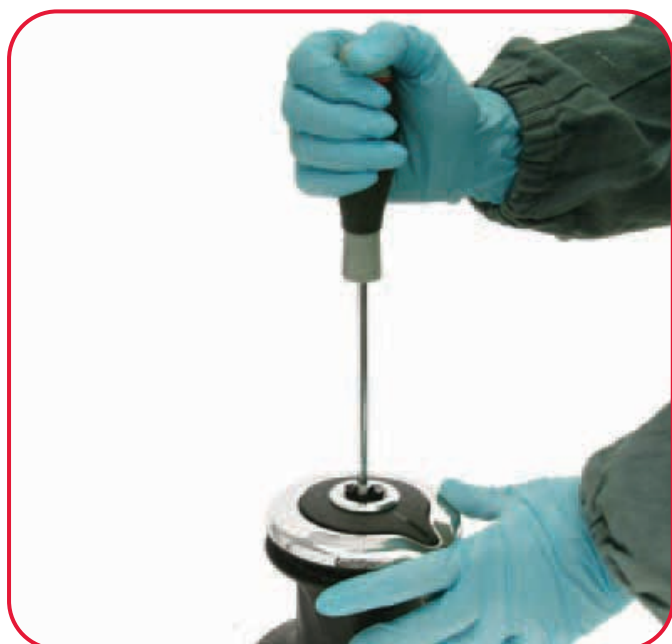
1. Unscrew the central screw ( 2 Nm/18 in-lb)
