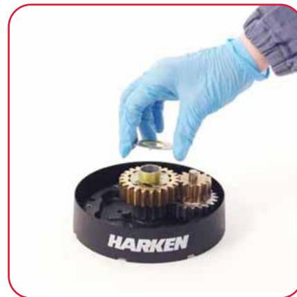
12. Remove the washer. Important: washer may remain inside the drum support!
