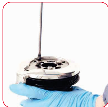
3. Unscrew the three screws (4Nm/35in-lb)
