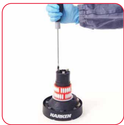
7. Completely unscrew three screws
