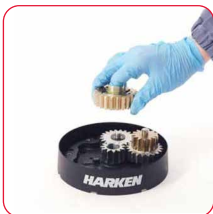
13. Remove the gear and remove the pawls. To facilitate the operation press the spring against the pawl with a blade.
