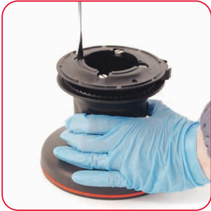
1. Unscrew the four screws (4 Nm/35 in-lb)
