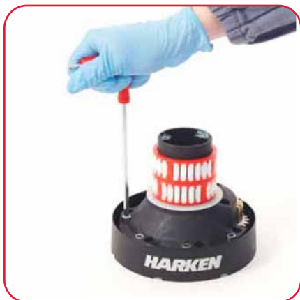
10. Unscrew the 6 stainless hex screws (8 Nm/71 in-lb) NOTE not those painted red
