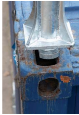
Place container post into ISO corner casting
