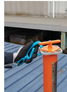
Attach hook on SRL to anchor point on container post
